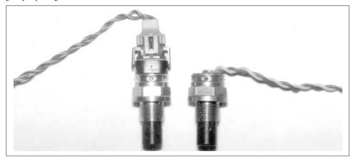
This shows a closer view of the modified speed sensor, compared to the stock sensor (GM part # 15547452, used on 1989 and newer 4X4 trucks) and wiring connector. You can modify the speed sensor yourself if you are good with a soldering iron, or the modified speed sensor (with 18" of wiring) is available from Stealth Conversions as part # 4L60-015.
