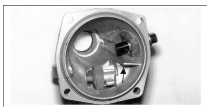
The location of the speed sensor is important so as not to block the rail (arrow) that is designed to allow oil to flow to the rear bushing (Prototype tailhousing shown).
